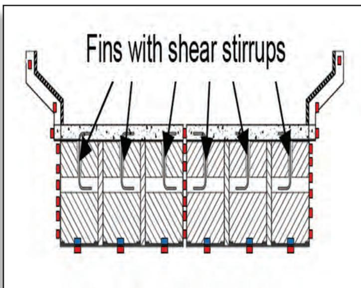
In addition to the HCB technology, this span also features an innovative, lightweight, modular polymer concrete ballast curb design. To date, the ballast curbs are also performing well. These lightweight ballast curbs contribute significantly to weight reduction.
